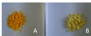
Figure 3 A - the raw CoQ 10 and B - powder of lipid-free CoQ 10 nanosuspension stabilized by TPGS
